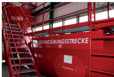
The 14-metre-long simulator at our training centre allows operatives to practise using their RPE in a variety of environments
