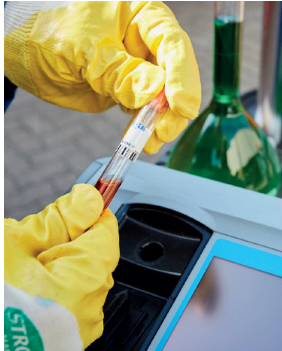
Regular analyses are conducted during the cleaning process. We check pH values, acid concentrations, iron content, conductivity and inhibitors in the mobile laboratory
